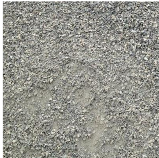
Cartpath gravel forms a hard surface that is suitable for active transportation. 3/8in Cartpath material example shown on the Mission Creek Greenway in Kelowna BC. Images Retrieved from: https://www.hikinqaddiction.ca/trails/viewtrail.php?trail_id=11 &
